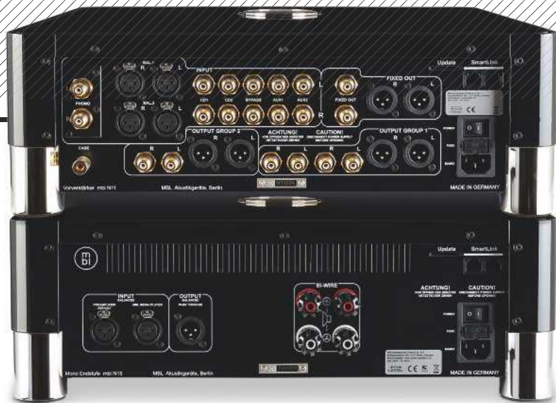
ABOVE: The N11 [top] has optional phono and seven line ins (two on XLRs and one HT/AV bypass) and three groups of preamp outs – fixed on XLR/RCA plus variable on XLR/2x RCAs and XLR/1x RCA. N15 [one shown, bottom] has XLR inputs, a loop-through line output plus two sets of 4mm WBT 'full copper' cable posts
