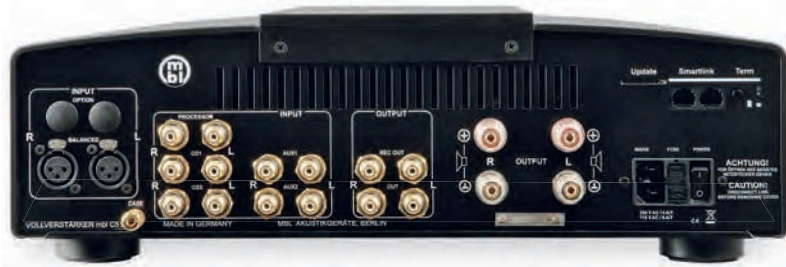
ABOVE: As with the Corona Line C31 CD player/DAC, on the rear panel of the C51 there's an integrated SD card reader slot for uploading any future software updates. Blanking plates allow the fitting of an additional XLR input or optional phono stage
