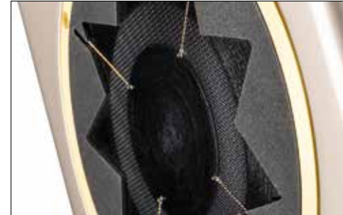
Different frequencies set different parts of the membrane into vibration. That's the design principle of the Manger transducer.
