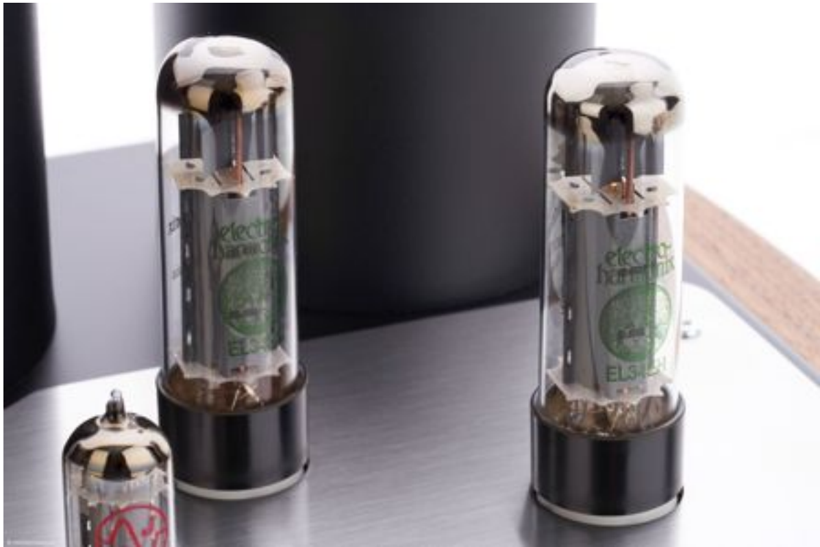
The two EL34s work in parallel in single-ended mode
